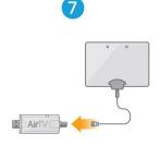
**Connect AirTV Adapter**... to your antenna using a coax cable (not included).
